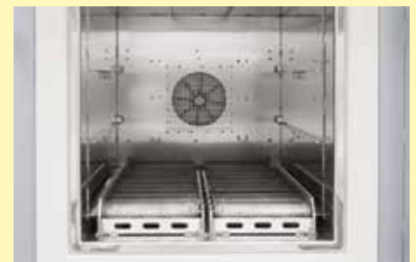
Roller conveyor in furnace chamber
