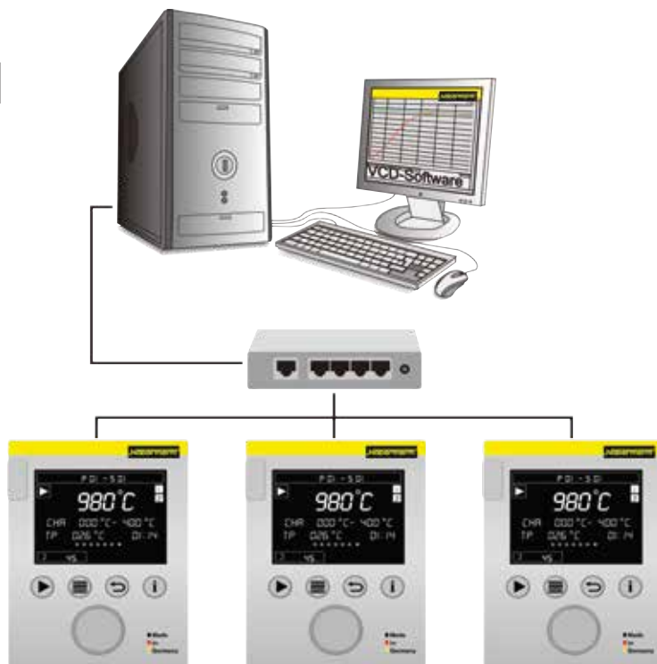
Example lay-out with 3 furnaces
